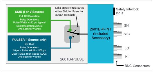
External Interlock/Connector box included with 2601B-PULSE
